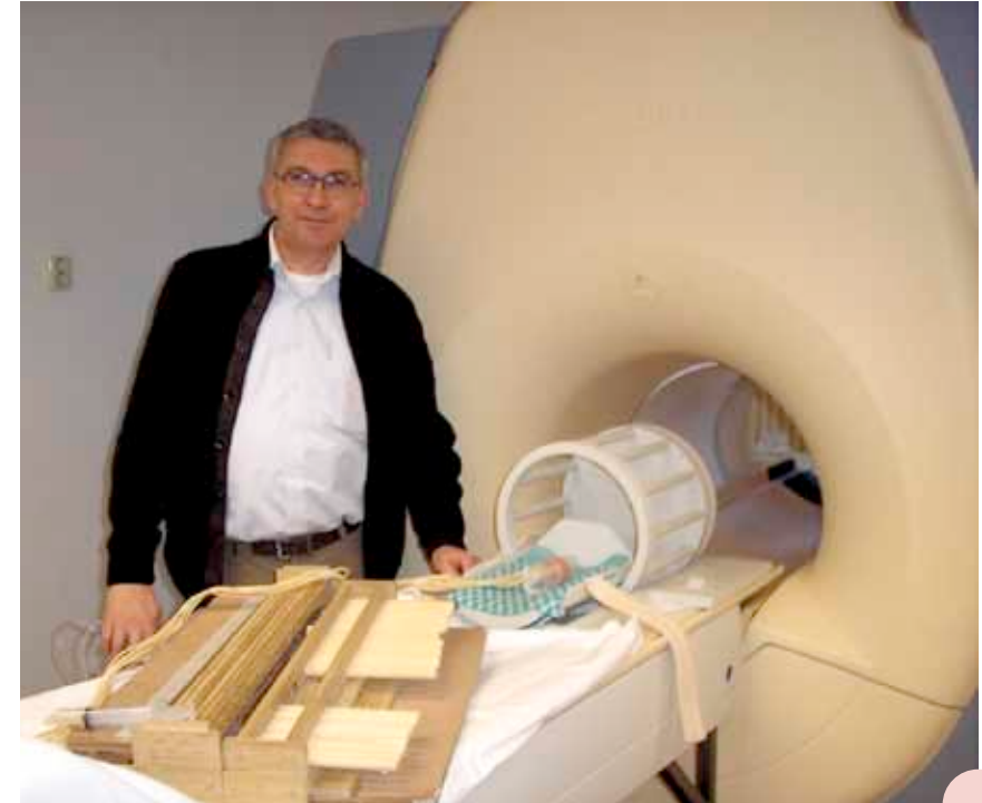
Prof. Gert ter Horst with an fMRI compatible device to feed people in the fMRI scanner. Luca Nanetti developed this device for his work characterizing the neuronal circuitry underlying appreciation of food products in healthy volunteers at the Neuroimaging Center in Groningen.
